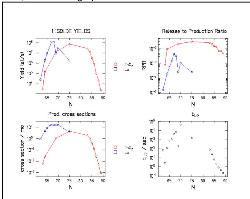
Fig.8: Results for I (Z=53) produced with ThO(red symbols) and La(blue symbols) targets
