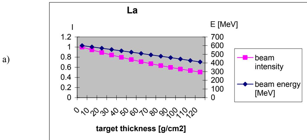
Fig.2: Energy and Intensity loss of a proton beam:
