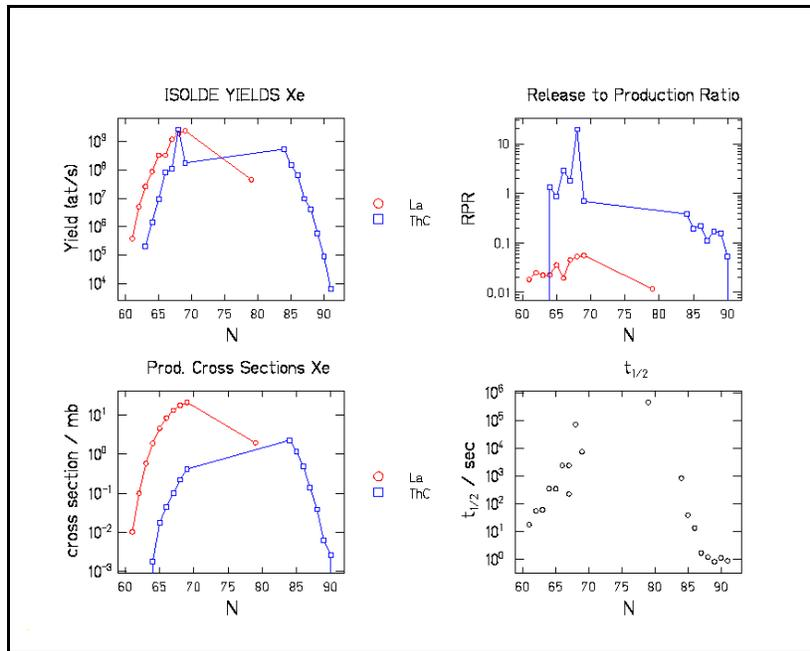
Fig.9: Results for Xe (Z=54) produced with La (red symbols) and ThC (blue symbols) targets
