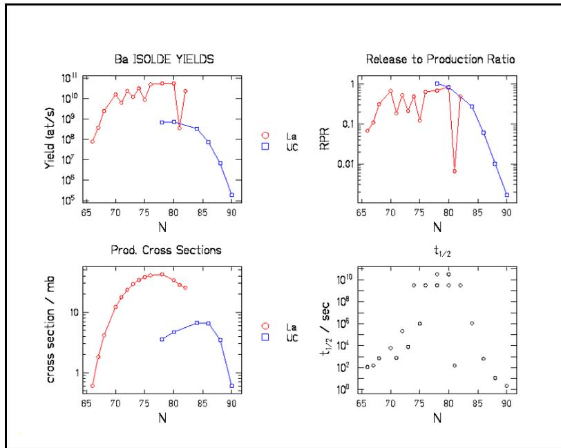
Fig.11: Results for Ba (Z=56) produced with La (red symbols) and UC (blue symbols) targets
