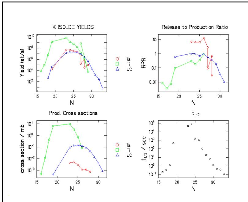
Fig.5: Results for K (Z=19) produced with Ta (red symbols), Ti (green symbols) and UC (blue symbols) targets
