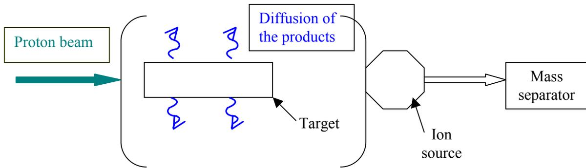
Fig.1: Scheme of the ISOLDE facility.
