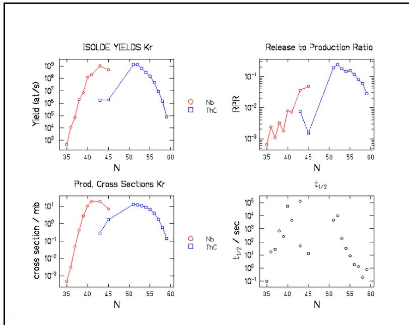
Fig.7: Results for Kr (Z=36) produced with Nb(red symbols) and ThC(blue symbols) targets
