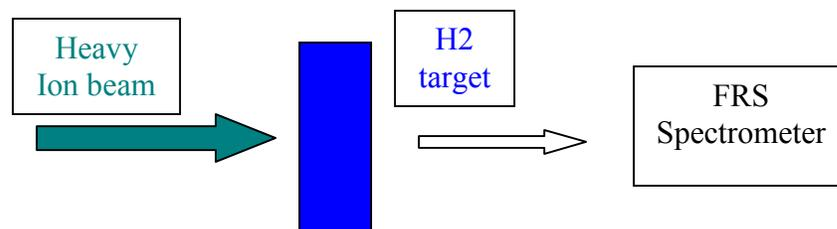
Fig.3: Scheme of the experiments in inverse kinematics at GSI.
