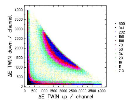
Figure 4: Cluster plot of fission fragments recorded by the double ionization chamber in the reaction  $^{238}\text{U} + (\text{CH}_2)_{n}$ .
