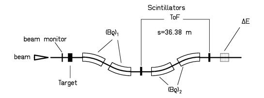
Figure 1: Schematic presentation of the fragment separator and the main detectors.
