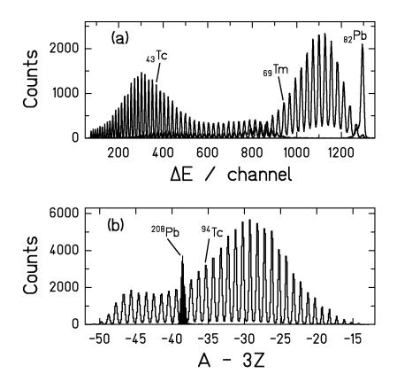
Figure 2: Example for the resolution in nuclear charge and mass for reaction products of the system  ${}^{1}\text{H} + {}^{208}\text{Pb}$  at 1*A* GeV (from Reference [8]). The spectra measured with a few different settings of the spectrometer are overlaid.
