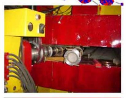
~5-10<sup>13</sup> protons are required for irradiating each of 55 targets to measure 10min - 30 years lifetime nuclides. This will take ~ 300 hours of accelerator operation time.
