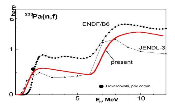
The predicted cross-section of <sup>233</sup>Pa(n,f) reaction.
