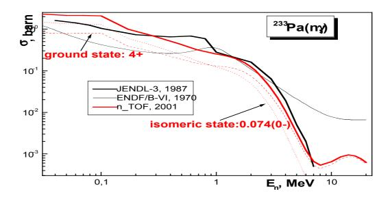
The cross-section of  $^{233}$ Pa(n, $\gamma$ ).
