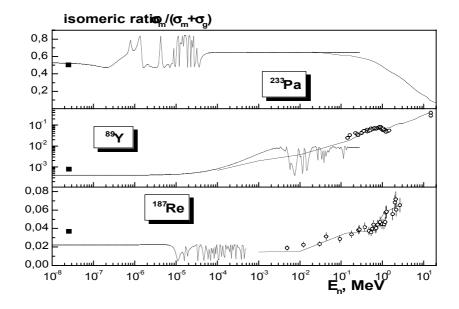
Isomeric ratios of neutron radiative capture by <sup>187</sup>Re, <sup>90</sup>Y and <sup>233</sup>Pa nuclei. Curves – calculations on the basis of the statistical model with account for
