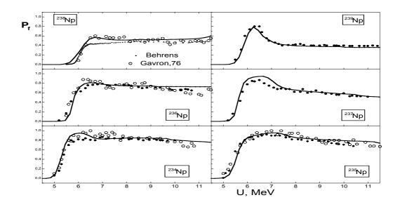
Fission probabilities of neptunium isotopes in dependence of excitation energy of fissioning nucleus from the reactions (<sup>3</sup>He,df), (<sup>3</sup>He,tf) \_ (n,f). Points- experimental data from [6.7], curves – results of calculation.
