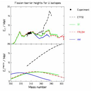
Figure 1: Full macroscopic-microscopic (upper part) and macroscopic part (lower part) of the fission barrier calculated for different uranium isotopes using the models mentioned in the text.
