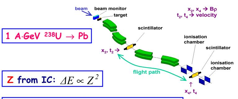
A/Z from time and position:  $\frac{A}{Z} = \frac{e}{m_0} \frac{B\rho}{c\beta\gamma}$
