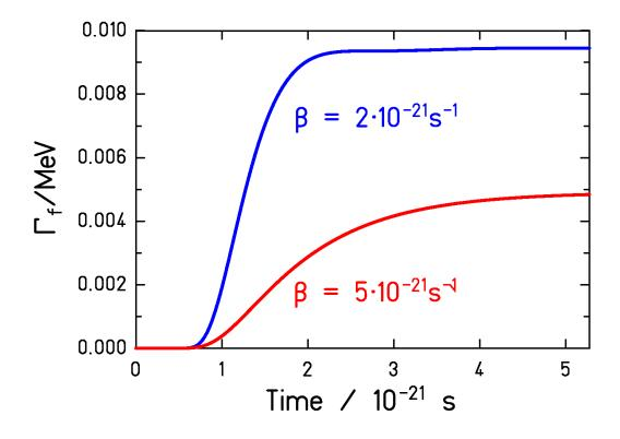
An example for the solution of the Fokker-Planck equation used in the nuclear-reaction code.
