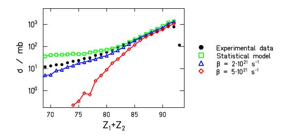
Fission of <sup>238</sup>U (1 A GeV) in a plastic target.
