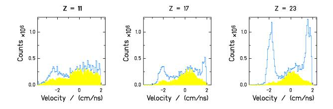
Residue production by <sup>238</sup>U (1 A GeV) + Ti (yellow) and <sup>238</sup>U (1 A GeV) + H (blue)
