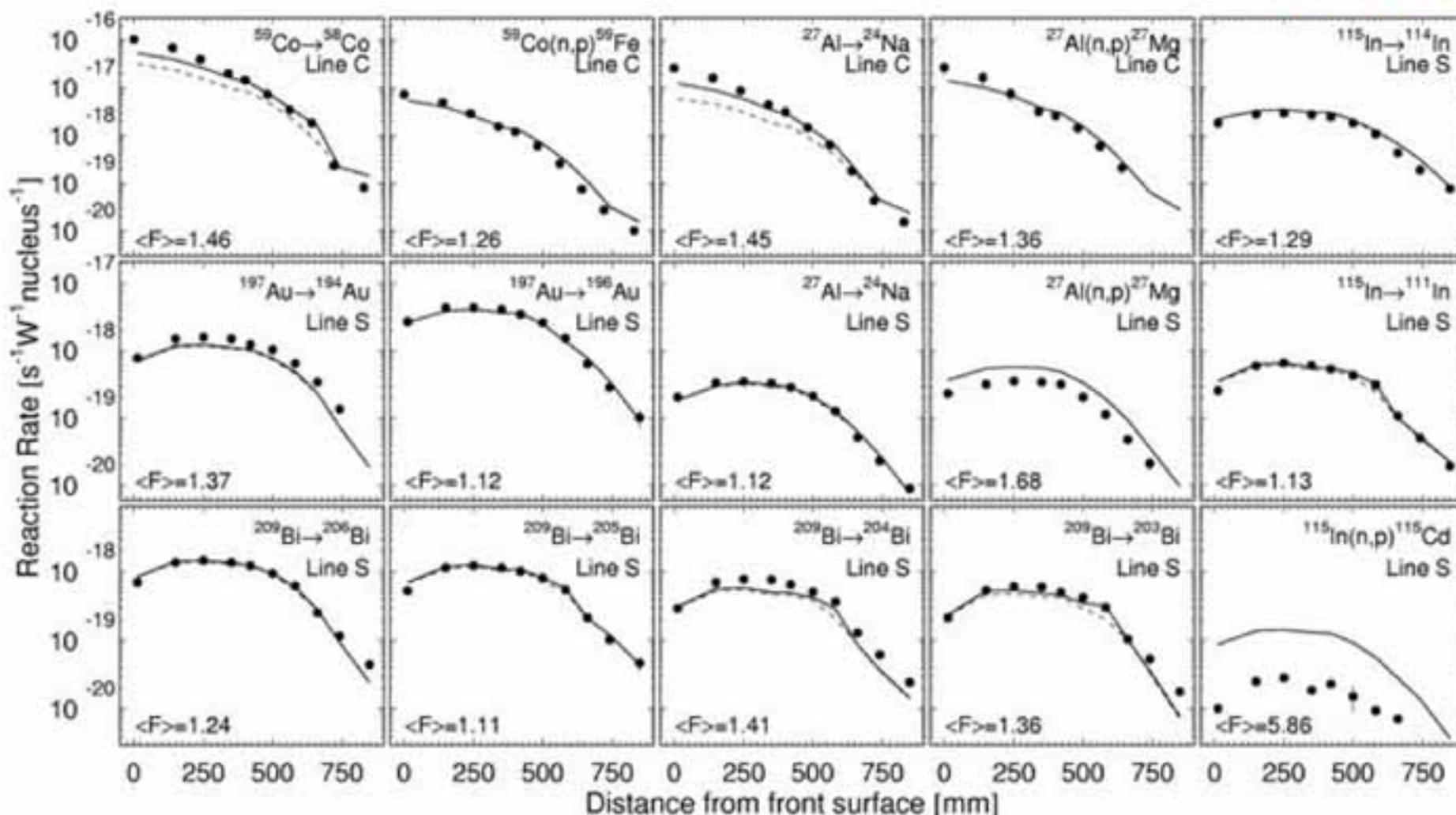
Reaction rates on W-Na thick targets irradiated with 0.8 GeV protons:
