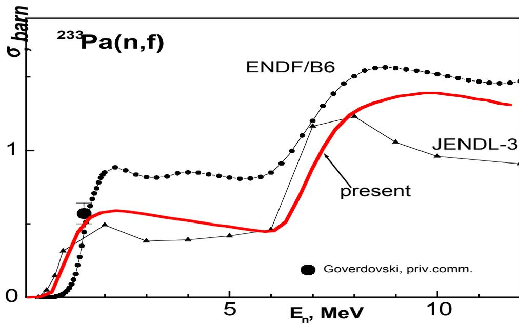
The predicted cross-section of  $^{233}\text{Pa}(n,f)$  reaction.
