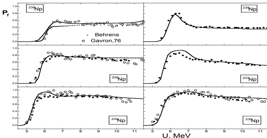
**Fission probabilities of neptunium isotopes in dependence of excitation energy of fissioning nucleus from the reactions  $(^3\text{He},df)$ ,  $(^3\text{He},tf)$  \_  $(n,f)$ . Points- experimental data from [6.7], curves – results of calculation.**
