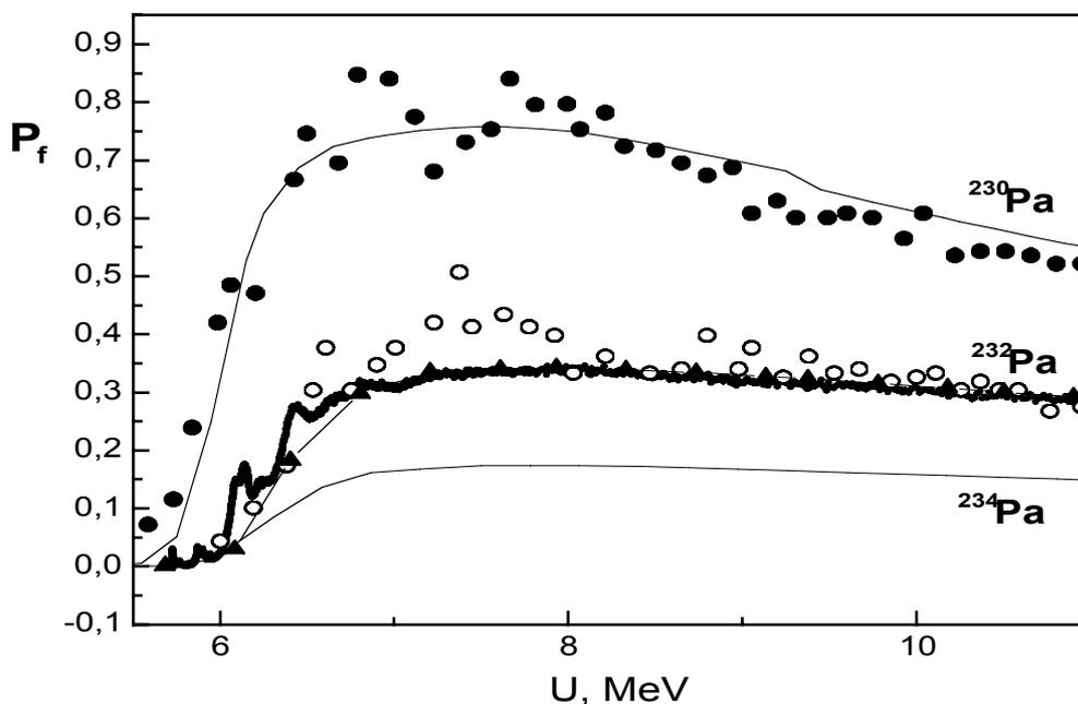
**Fission probabilities of the odd-odd Pa isotopes in dependence of excitation energy of fissioning nucleus Points – experimental data from [6.7], curves – results of present calculation.**
