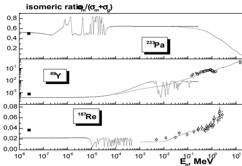
Isomeric ratios of neutron radiative capture by  $^{187}\text{Re}$ ,  $^{90}\text{Y}$  and  $^{233}\text{Pa}$  nuclei.
