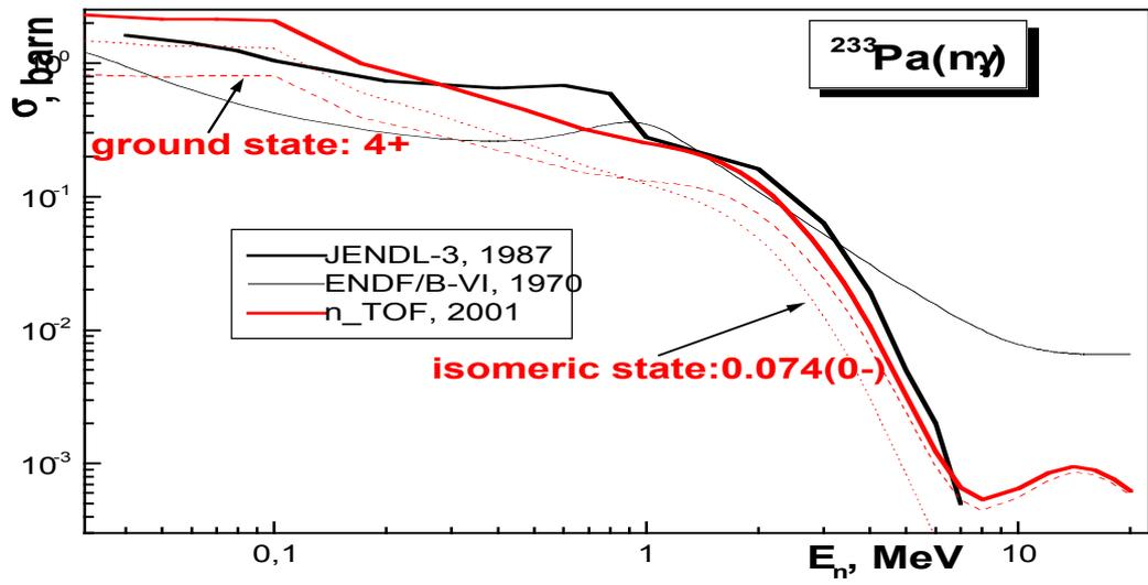
The cross-section of  $^{233}\text{Pa}(n,\gamma)$ .
