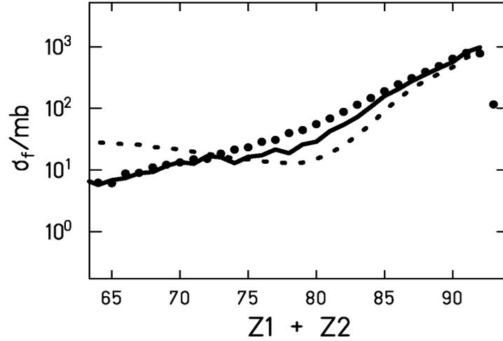
**Figure 6:** Experimental partial fission cross sections for  $^{238}\text{U}$  impinging on  $\text{CH}_2$  at 1 A GeV (full dots) in comparison with two calculations. The full line corresponds to a calculation done with  $\Gamma_f(t)$  as a step function and  $\beta = 2 \cdot 10^{21} \text{ s}^{-1}$ , and the dotted line to a calculation with  $\Gamma_f(t) = K \cdot \Gamma^{\text{BW}}(1 - \exp(-2.3 \cdot t / \tau_f))$  and  $\beta = 9 \cdot 10^{21} \text{ s}^{-1}$
