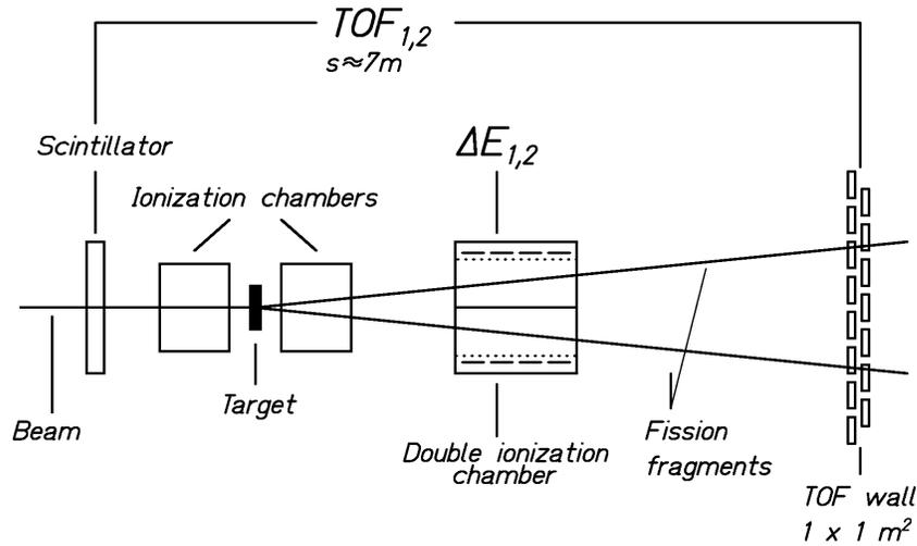
**Figure 3:** Experimental set-up for fission studies
