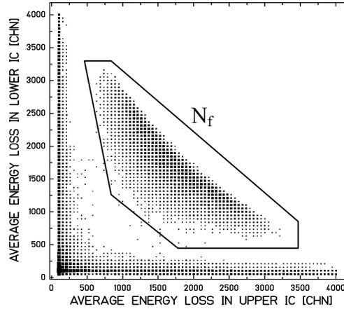
**Figure 4:** Scatter plot of the energy loss signals in the double IC. The applied condition selects the fission events  $N_f$ .
