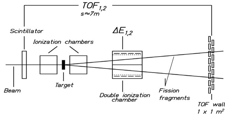
FIGURE 2. Experimental set-up for fission studies
