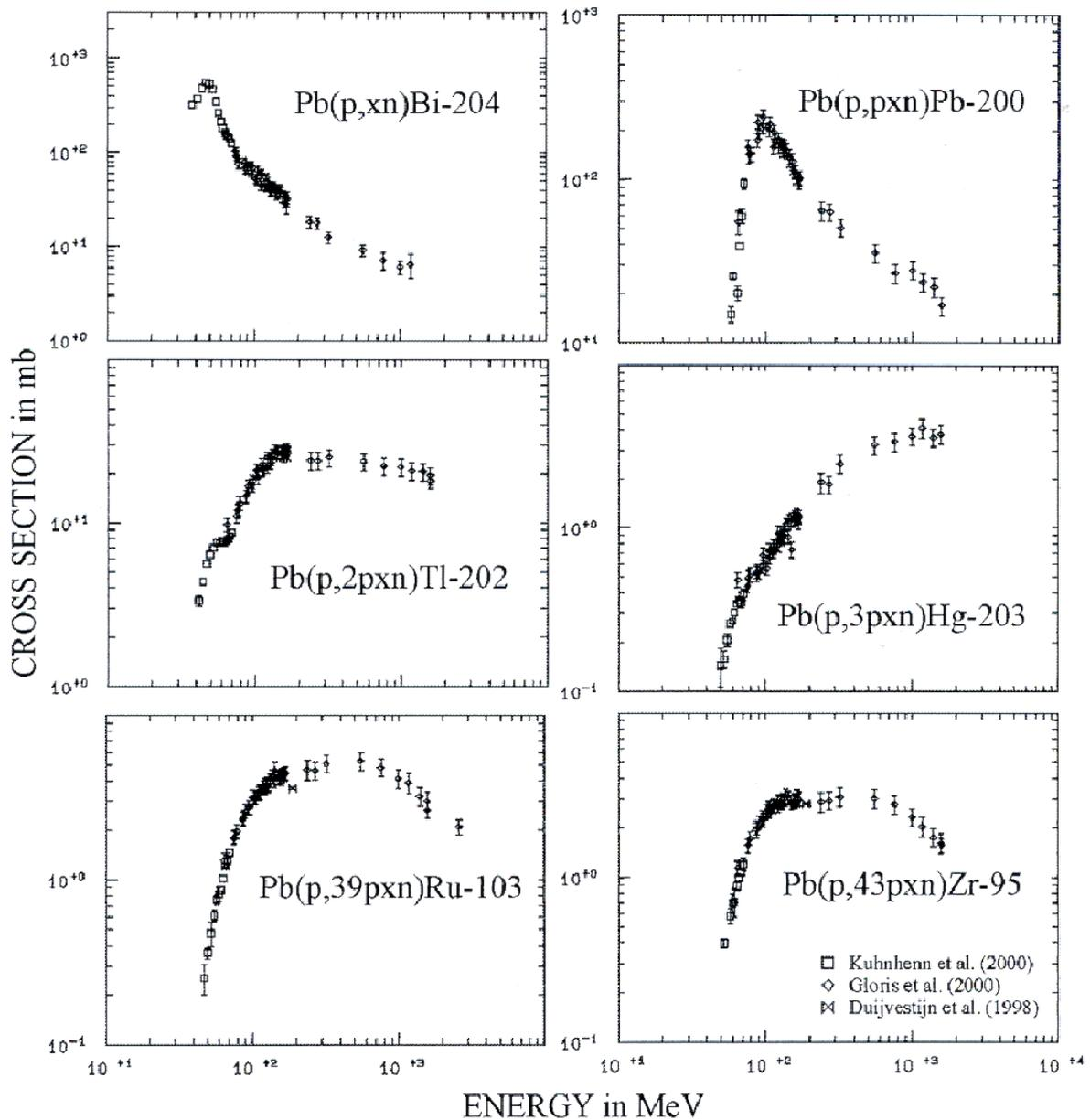
Excitation functions for some selected isotopes produced in the interaction of protons with lead.
