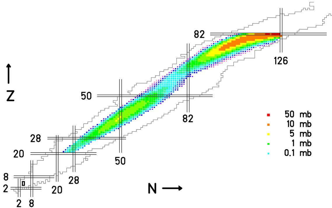
Cross sections of heavy residues measured in inverse kinematics.
