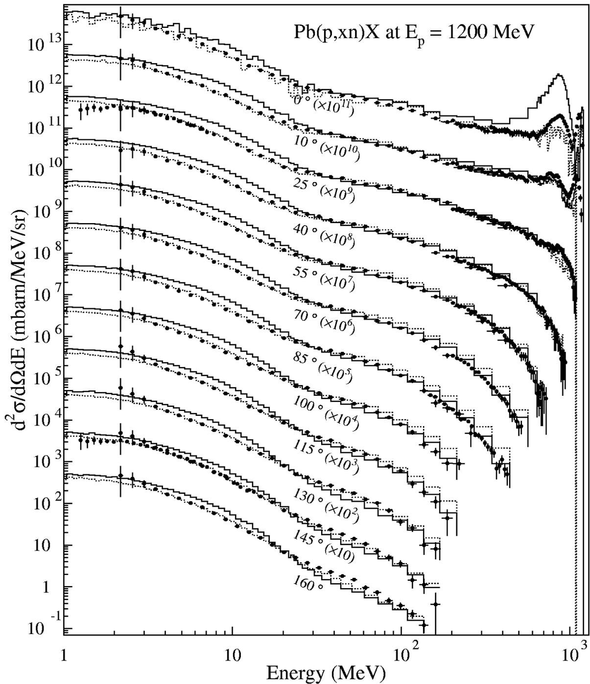
Neutron production double-differential cross sections. Data points with Bertini INC (histograms) and Cugnon INC (dotted lines).
