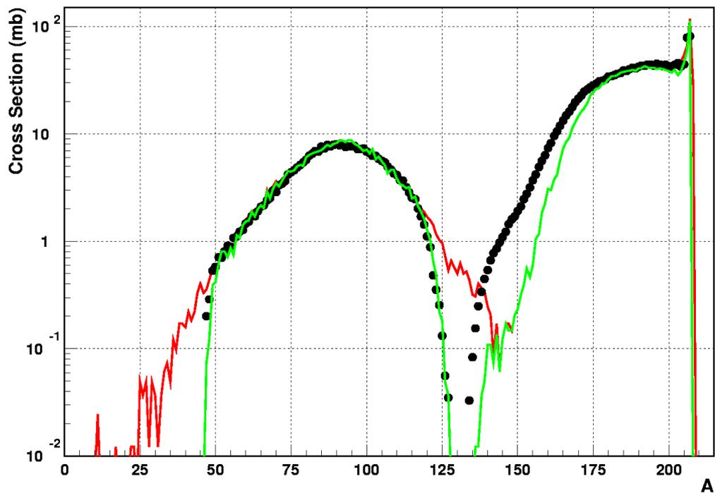
Data points (T. Enqvist et al.) in comparison with calculations of total production (red line) and that of measured nuclides only (green line).
