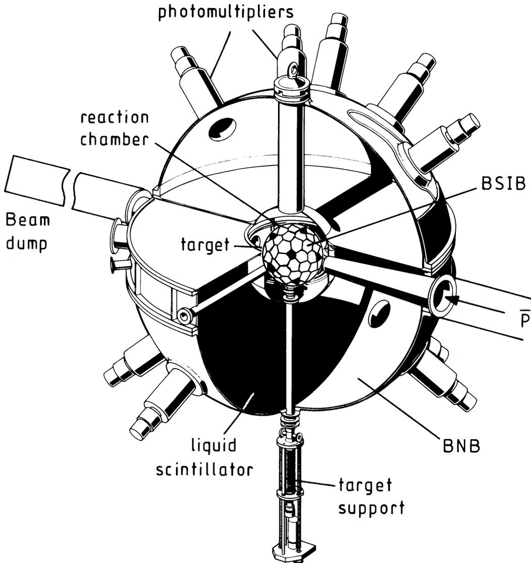
**A  $4\pi$  detector for neutrons and charged-particles**
