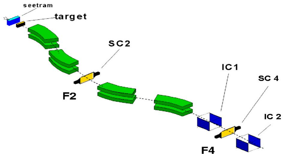
After identification of  $Z$  and  $A$  ( $Z$  and  $A$  are integer numbers)  $B\rho$  provides velocity with high precision  $\rightarrow$  resolution of  $5 \cdot 10^{-4}$  in  $\beta \cdot \gamma$ !
