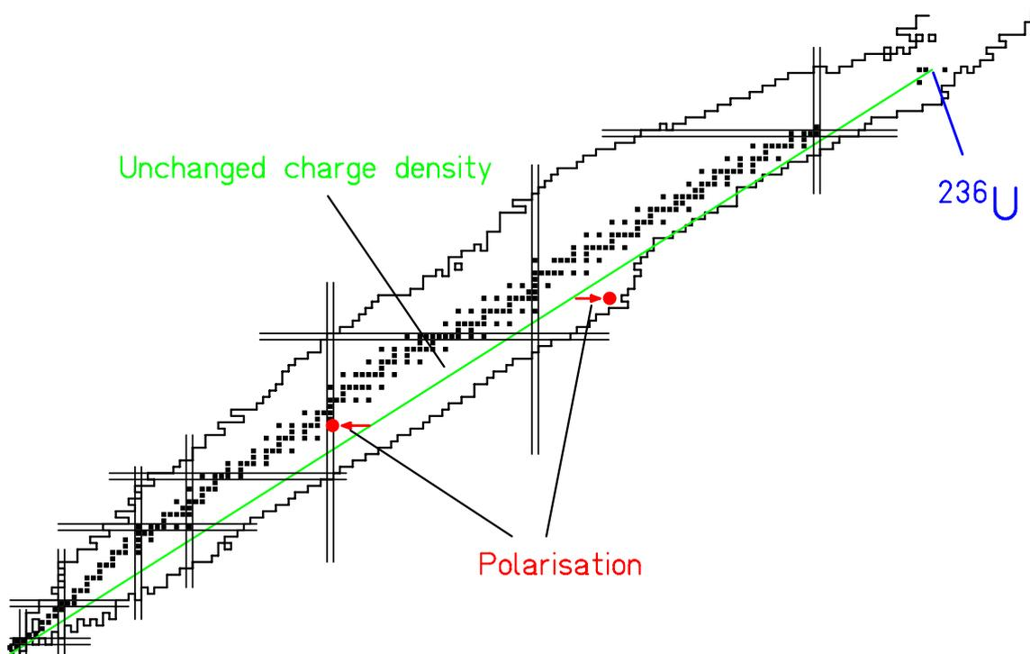
Charge polarisation (variation of the N/Z ratio of the fragments) is the only way to exceed the N/Z of the fissioning system.
