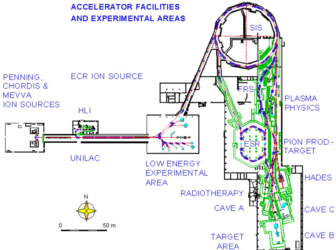
Heavy nuclei ( $^{197}\text{Au}$ ,  $^{208}\text{Pb}$ ,  $^{238}\text{U}$ ) are accelerated and hit the production target. The projectile-like residues are identified in-flight with the fragment separator (FRS).
