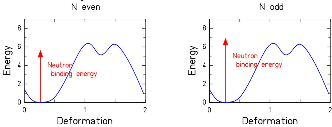
**Only nuclei with odd neutron number fission after capture of thermal neutrons, energy release  $\approx 200$  MeV.**
