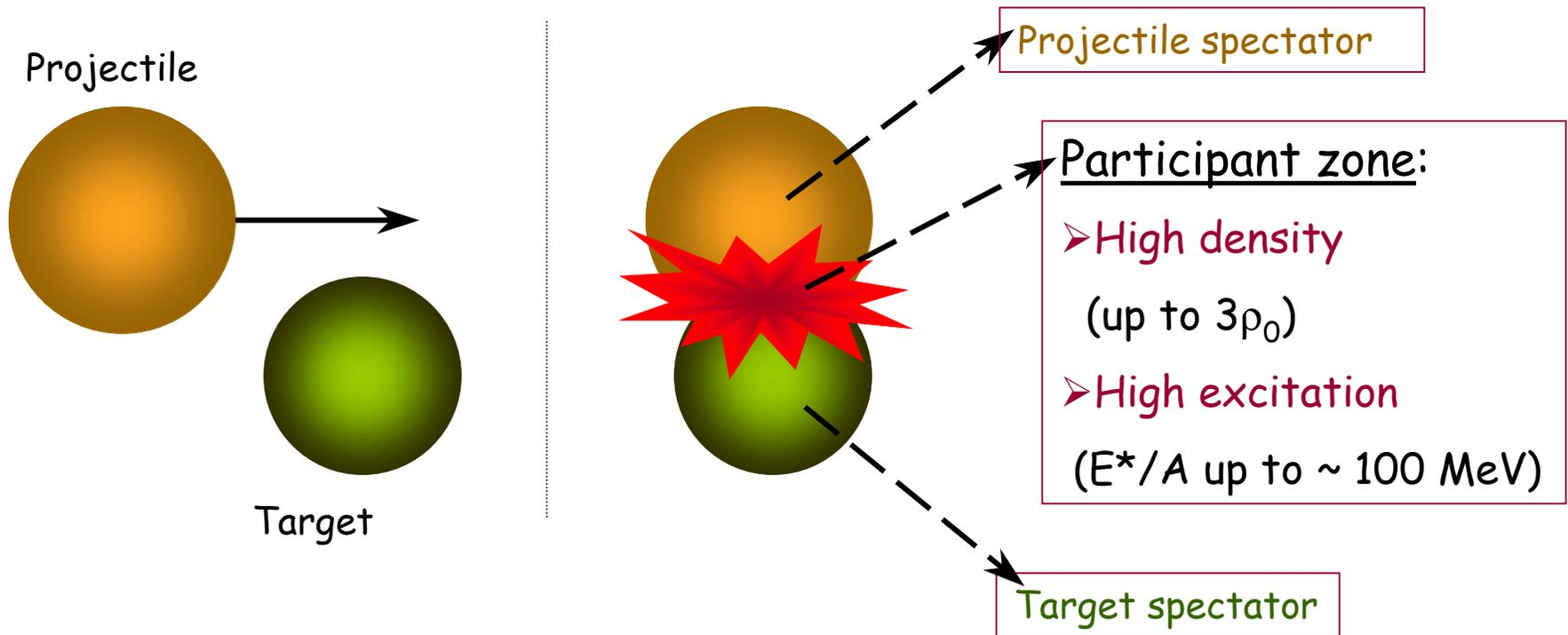
➤ "Standard" experiments: Detection of nucleons, produced particles, very light fragments in large-acceptance experiments.
