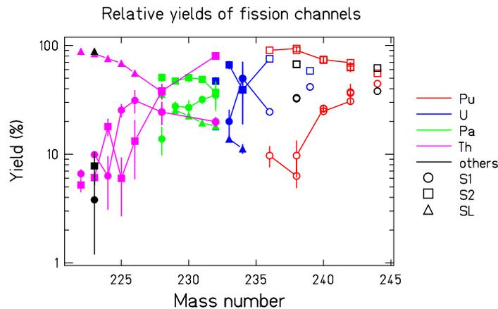
Fig. 2. (Color online) Relative yields of the three independent fission channels Standard I (S1), Standard II (S2) and Super long (SL). For reference to data, see Appendix of Ref. <sup>2</sup>. All data are given in mass numbers. Values measured in nuclear charge were converted to mass numbers using the unchanged-charge-density assumption and neglecting neutron evaporation. The shape of the symbol marks the fission channel.
