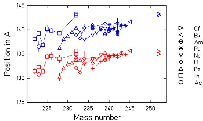
Fig. 3. (Color online) Mean positions of the three independent fission channels Standard I (S1), Standard II (S2) and Super long (SL). All data are given in mass numbers. Values measured in nuclear charge were converted to mass numbers using the unchanged-charge-density assumption and neglecting neutron evaporation. The shape of the symbol indicates the element. For reference to data, see text.
