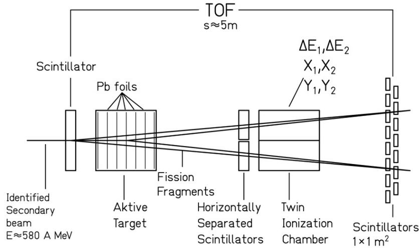
Fig. 1: Experimental set-up at the focal plane of the GSI Fragment Separator for the investigation of fission of secondary beams in inverse kinematics.
