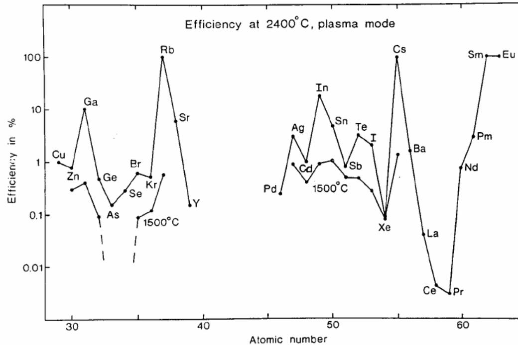
Fig. 13. The overall efficiency of the OSIRIS target and ion source as a function of atomic number of fission-product nuclei. The upper curve is measured at a target temperature of 2400°C. For comparison the lower curve shows the efficiencies of the previously used system at 1500°C.
