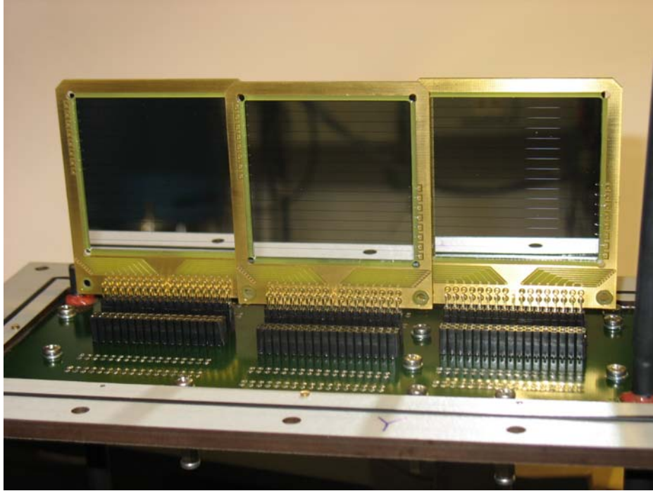
Fig. 3: The 'active catcher' of the present RISING campaigns consists of three Si strip detectors.
