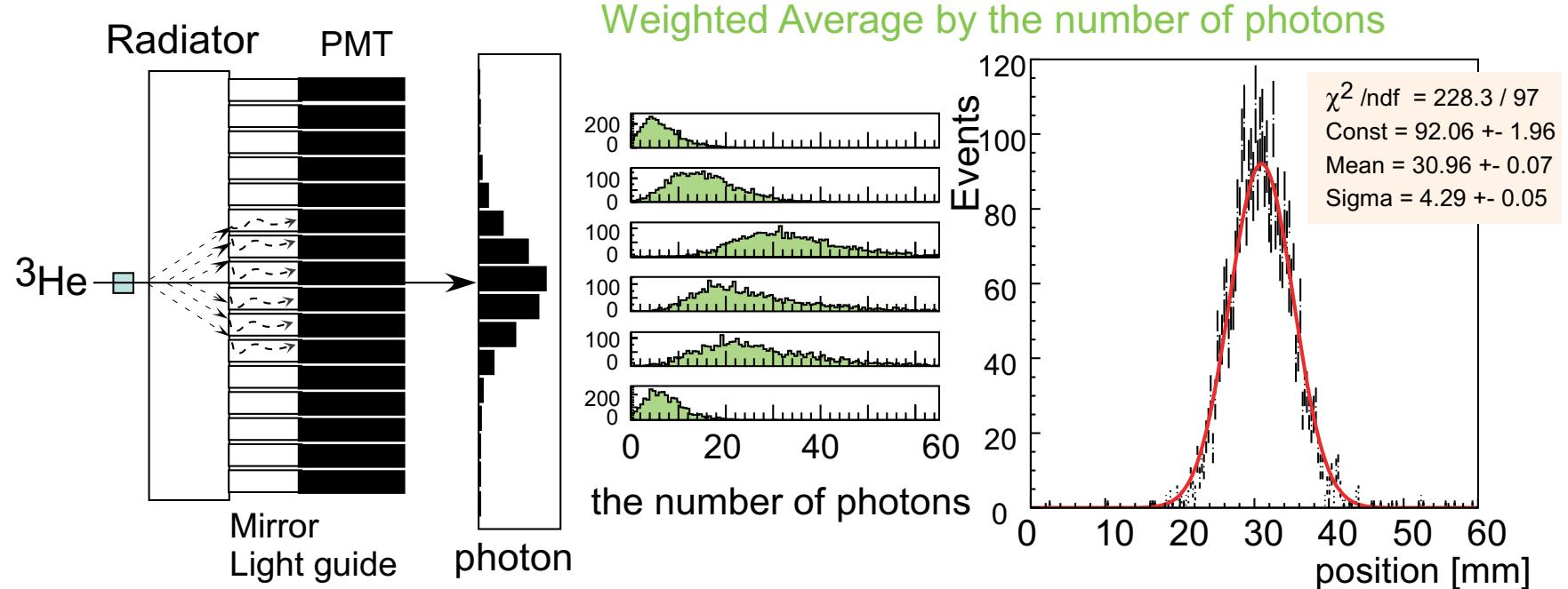
Position resolution of TORCH at S2  $\sigma \sim 4.5$  mm
