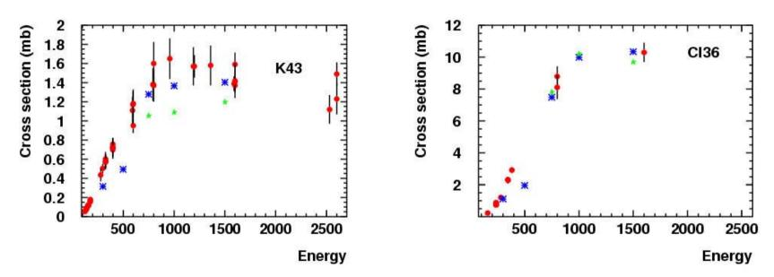
Excitation fonctions for two isotopes created in direct kinematics and detected by gamma spectroscopy (R.Michel et al. Nucl. Instr. Meth. Phys. Res. B 129 (1997) 153-193 Good agreement, in general, at high energies for the 14 available isotopes.
