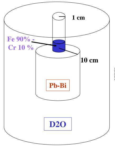
Chemical elements created in a window Fe 90% - Cr 10 % after one year of irradiation by a 31.8  $\mu A$  /cm<sup>2</sup>proton beam at 1000 MeV.
