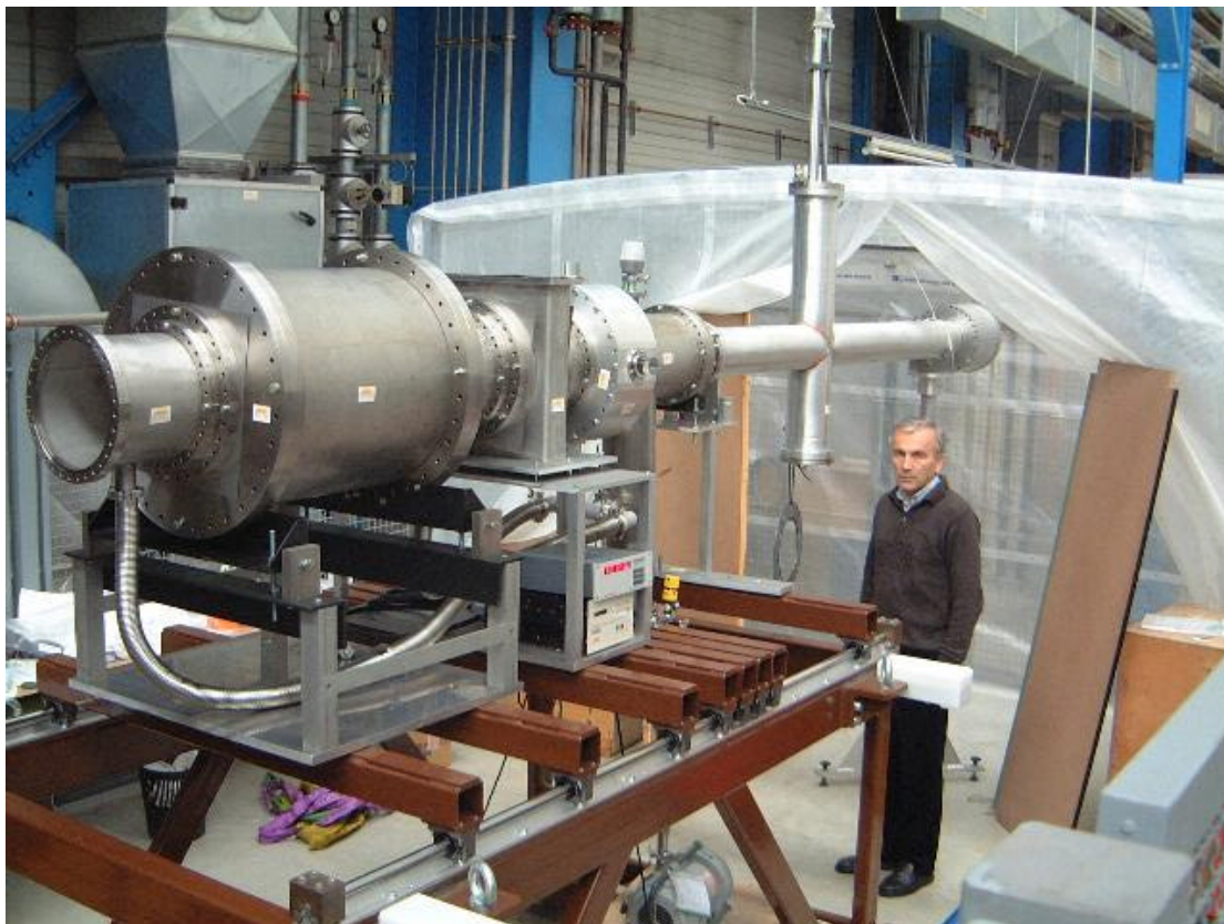
Fig. 3: Technical drawing and photo of the RISING beamline for experiments at relativistic energies
