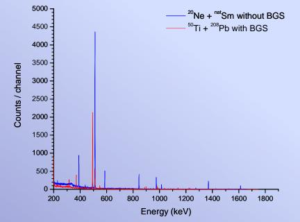
Direct catch measurement of nuclides produced in the <sup>nat</sup>Sm(<sup>20</sup>Ne,xn) reaction without pre-separation.
