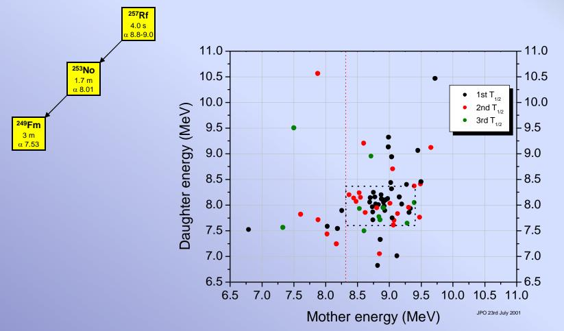
Correlation plot of  $\alpha$ -events detected in the <sup>257</sup>Rf - <sup>253</sup>No energy region during a SISAK run in November 2000 at LBNL using the BGS.
