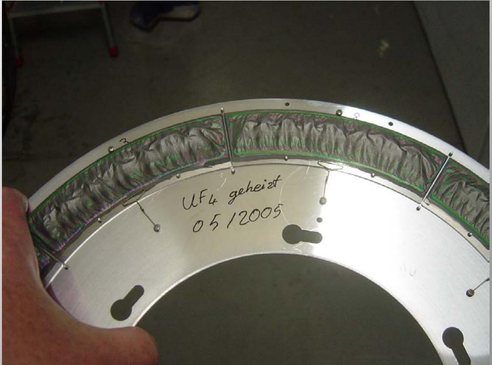
Rotating  $^{238}\text{UF}_4$  target wheel
