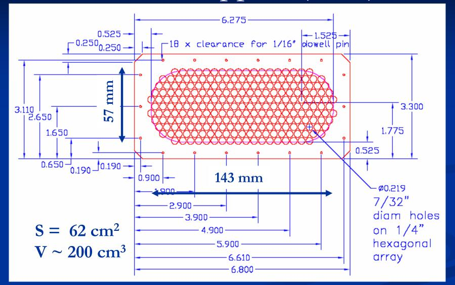
Hole diameter ~ 5.5 mm  $\rightarrow$ High transparency, but does not allow to work with Mylar < 2  $\mu$ m
