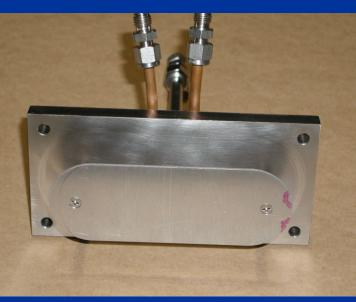
Thickness of Mylar foil : 2.5 µm Honeycomb mesh : 0.5 mm thick SS Transparency of mesh : 93 %
