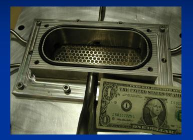
Smaller (fixed) volume Honeycomb grid allows thinner MYLAR Catcher foil holder for yield measurement
