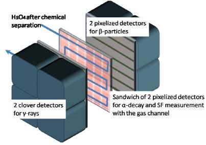
Figure. Proposed detector design for  $\alpha$ - $\beta$ - $\gamma$ -spectroscopy measurements of Hs nuclei and daughters.
