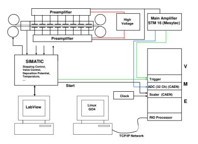
Figure 1: Schematic of the electrodeposition system with electrolysis cell, tape and detection system, the processor and data acquisition system
