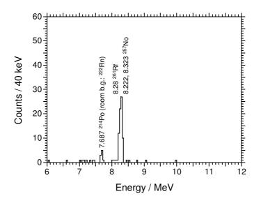
Figure 1. Sum of  $\alpha$ -particle spectra measured in the seven top detectors of MANON for 210 s after the 30-s aerosol collection. The 30-s aerosol collection was repeated 697 times. The beam dose of  $6.3 \times 10^{17}$  was accumulated.
